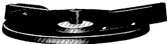
Fig. 2 a Normal broadcasting: Swivel blades in downward position "A"
