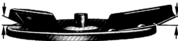
Fig. 2 b Late top dressing: Swivel blades in lifted position "B"
