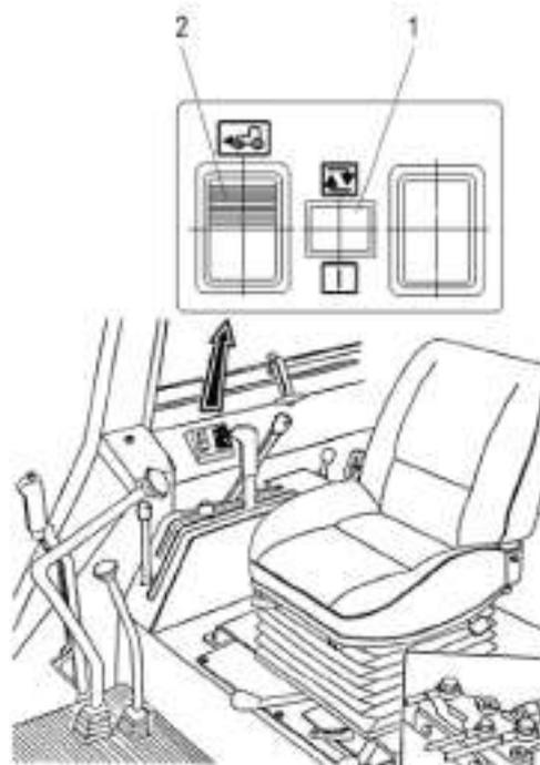
**Note:** The electric circuit of FDA drive control is provided with braking relay, ensuring automatic FDA drive switching on upon pressing interlocked wheel brake pedals. It is installed only on the models where FDA drive is aligned with DI.
