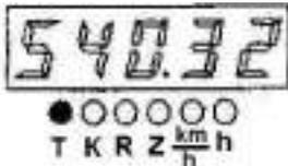
1) Transfer ratio of wheel reduction gear «K1»
