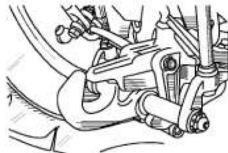
**Traction-coupling mechanism TCM-1M (pendulum)** — is used for operating heavy trailed machines (optional).
