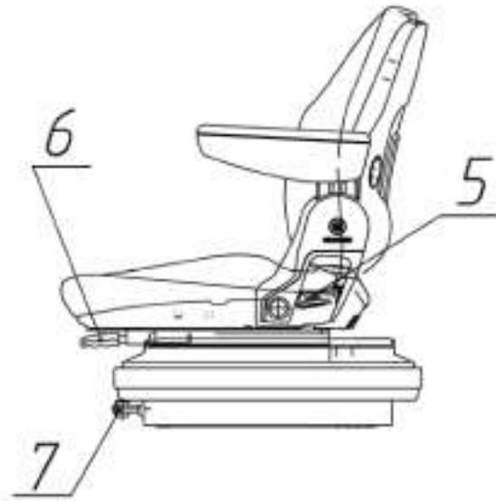
5—adjustment of seat-back tilt angle
